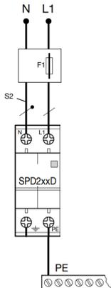
Overcurrent protection (F1) is provided by the upstream over current protection device (OCPD) which for a consumer unit is generally the service cut-out fuse.
